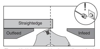
**Figure 13.** Using a straightedge to align outfeed table height with insert at TDC.
